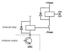
Fig. 4-31: Driving high-current loads
